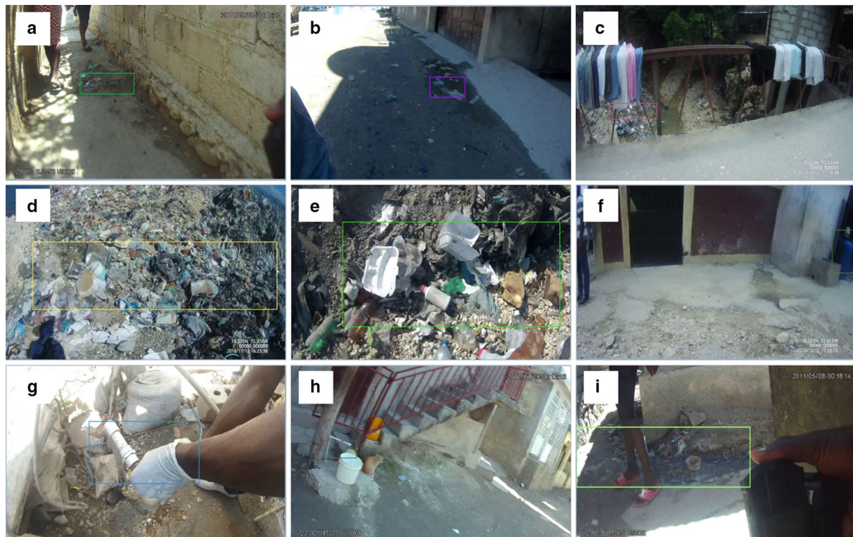
Fig. 11 Positive object detections after 3rd round of accuracy testing. The resolution for the image varied from 224 to 1280px. A frame window of 60 was selected for detection. Positive object detection examples for a Muddy Water (832px), b Muddy Water (1280px), c Trash (1280px), d Trash (416px), e Trash (416px), f Water Point (1280px), g Water Point (416px), h Water Point (1024px), and i Drain (416px)
